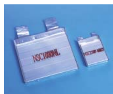
Next-generation condenser device (Original "ionic liquid" as electrolyte in capacitor)
