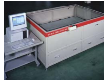
Our solar simulator to test the electrical performance of photovoltaic modules
