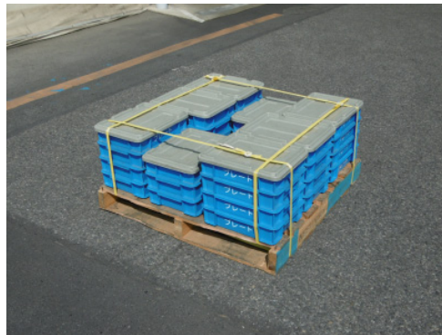
Bundling of incoming parts with PP bands (after improvement)
