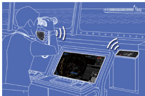
Call using wireless speaker microphone
