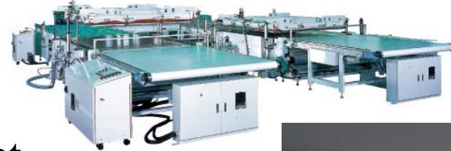
PV module laminators
