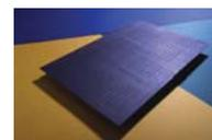
Carbon molded separator (bipolar plate)
