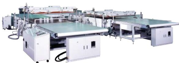
Solar Module Laminator, solar battery production equipment
