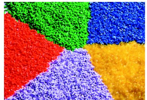
*Polyurethane elastomer pellet*
