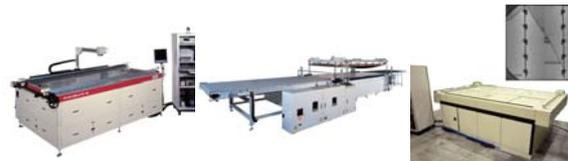
Photovoltaic module manufacturing line: a solar simulator (left), a module laminator (center), and an EL inspection unit (right)
