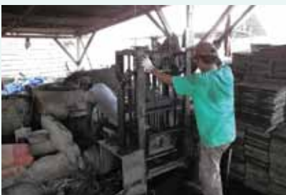
Turning coal ash into concrete blocks
