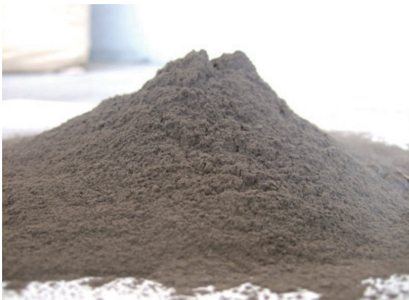
Shavings from grinding brake linings collected with a dust extractor (Toyoda Plant)
