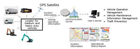
Connected services for commercial vehicles using locators for medium- and heavy-duty vehicles
